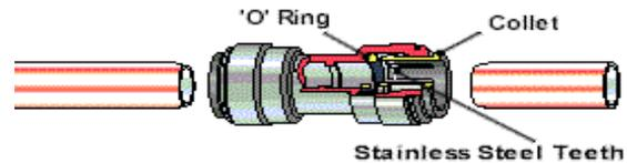
Cut the tube square. It is essential that the outside diameter be free of score marks and that burrs and sharp edges be removed before inserting into fitting.
